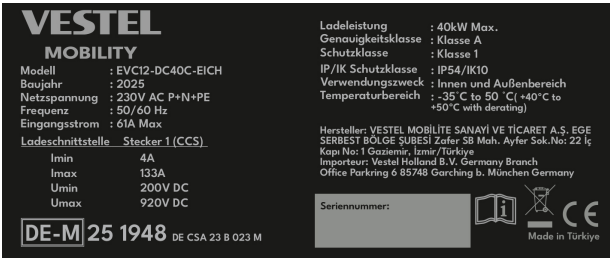
Example of a type plate for EVC12
