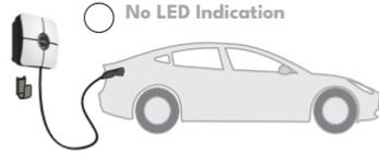
2- Insert the charging plug to the charging plug holder of the station.
