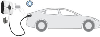
**Method 2.** You can terminate charging by unplugging the charging cable from the vehicle.
