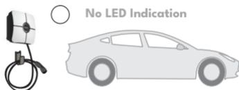
2- Insert the charging plug to the vehicle inlet.
